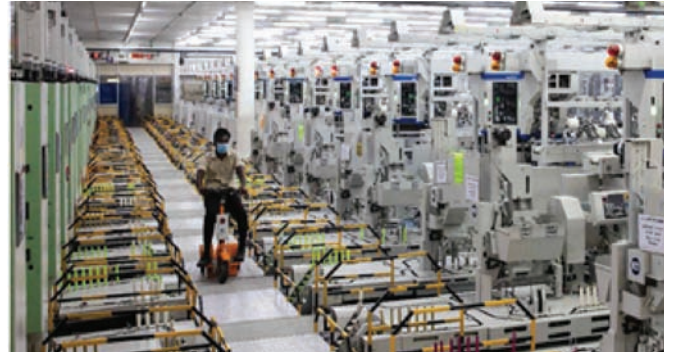
A view of most modern Ring Spinning Frames with link-coners installed at our Mills by replacing old machineries as a part of modernisation programme.
